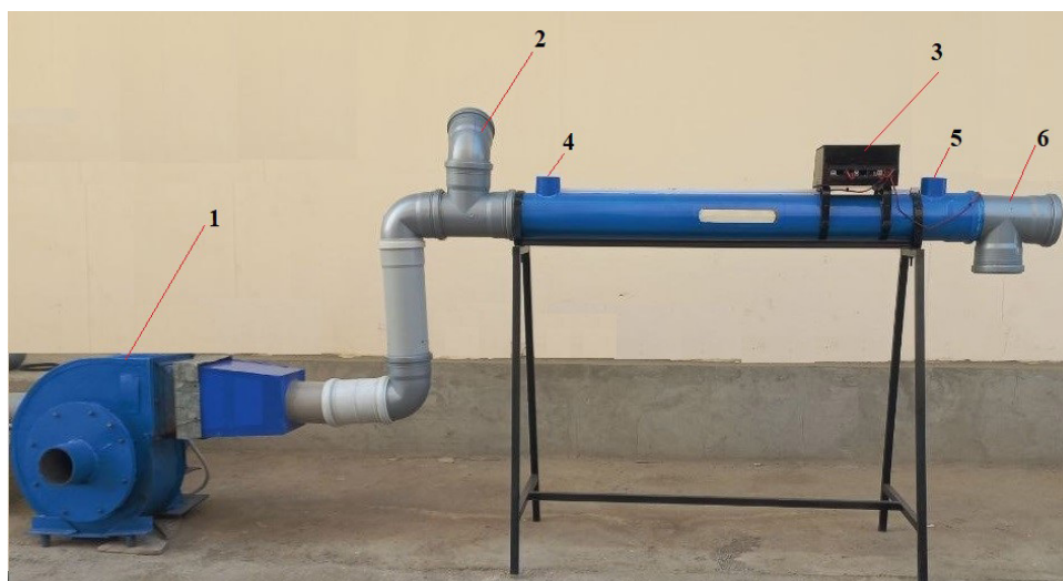
Photo/Figure 1. An experimental device for monitoring the parameters of factors affecting damage to cotton raw materials
